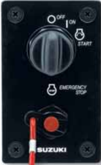
Single Engine Ignition and Emergency Stop Switch Control Panel
